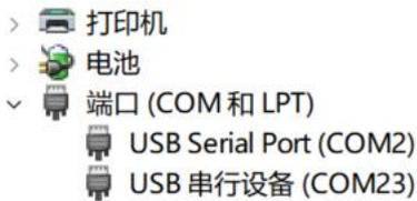
(2) Select the COM number by which the knob is recognized in the COM combo box. Then click "START" to initiate the download. After waiting for the "FINISH" prompt to appear in the status, unplug and replug the USB to perform a reset.
